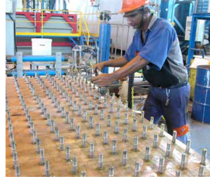
Refurbishment of copper-mold plates
