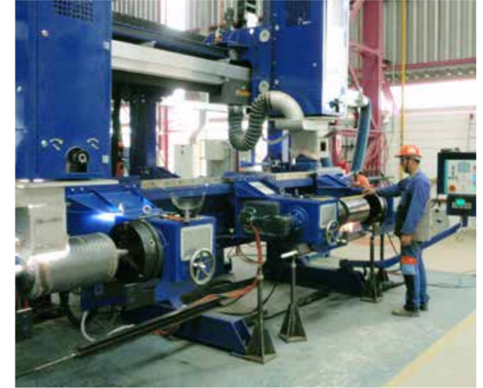
Roll cladding center developed by Primetals Technologies
