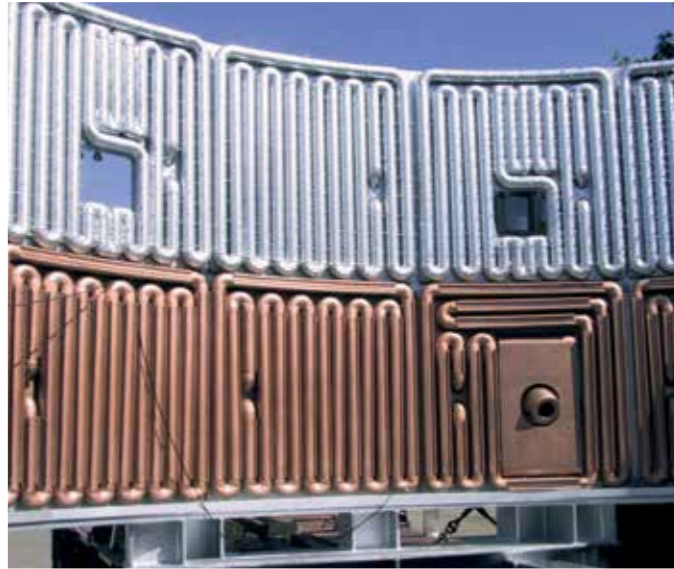
Electric arc furnace panel
